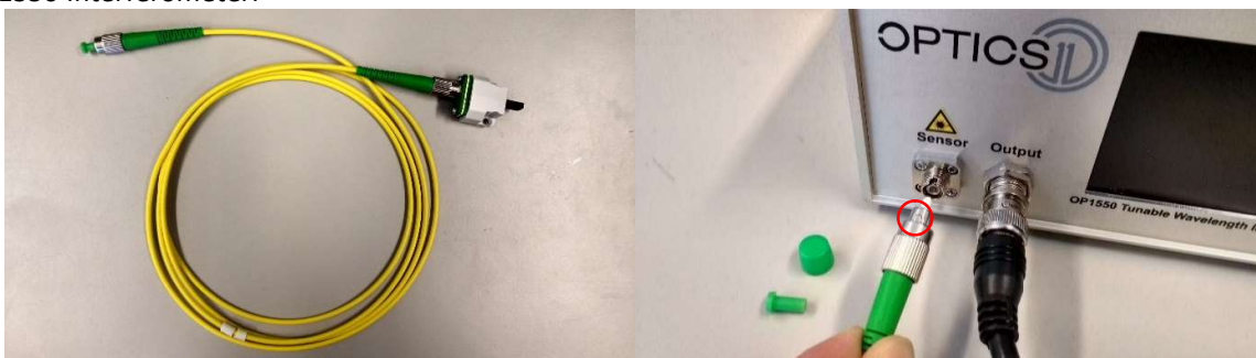
Figure 7: Connecting the left end of the patch-chord to the OP1550, a notch (red circle) indicates the preferred orientation
