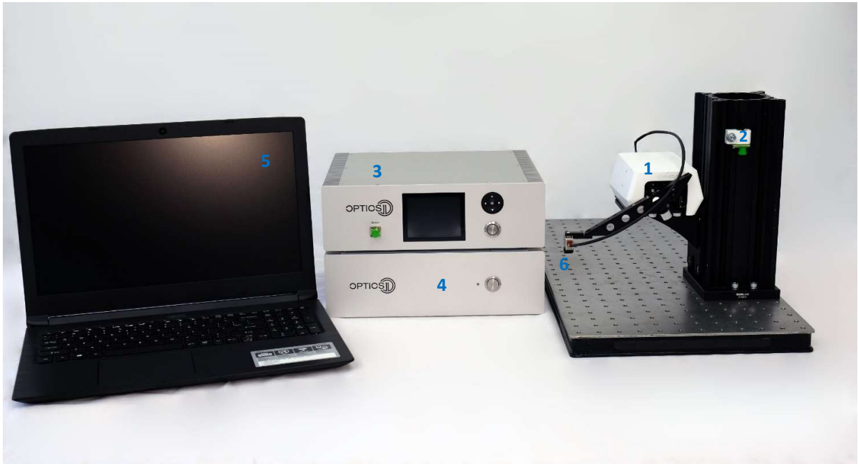
Figure 2: Picture of the Chiaro Nanoindenter setup showing the Chiaro indenter head (right), OP1550 interferometer, controller box, and PC.
