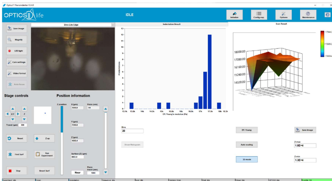
Figure 43: The scan results tab shows a 5x5 2D plot and a histogram.
