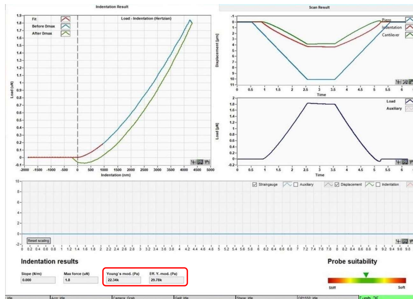
Figure 41: Indentation results after indenting a sample in D-mode.
