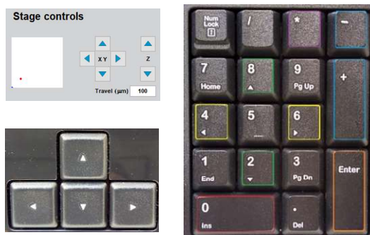
Figure 22: Keyboard stage controls (X stage, Y stage, Z+ up, Z+ down, Stop).
