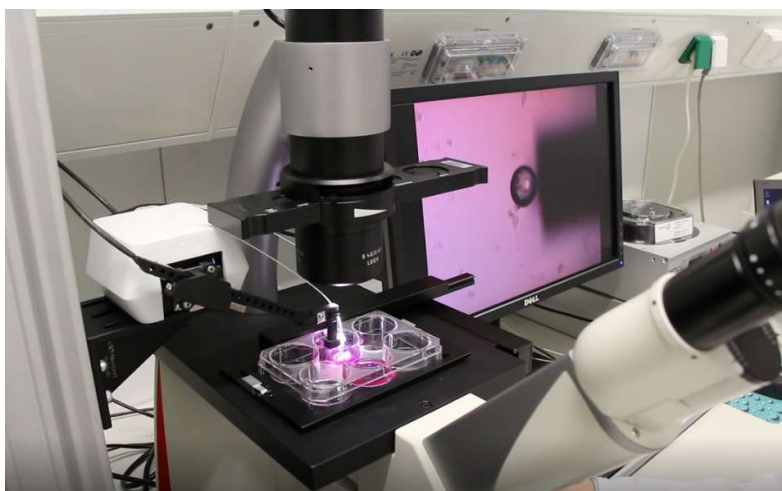
Figure 20: Example of calibrating the probe in a medium droplet on top of a regular microscope sample slide.
