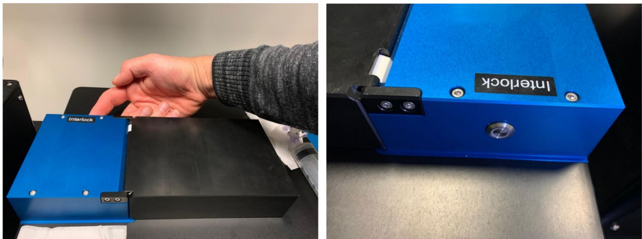
Figure 2. Interlock relay switch is located on the back side of the chamber lid.
