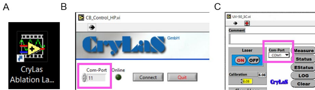
Figure 3. Starting CryLas software. Desktop shortcut for CryLas software (A). Com port input in newer software highlighted in magenta (B). Com port input in older software highlighted in magenta (C).
